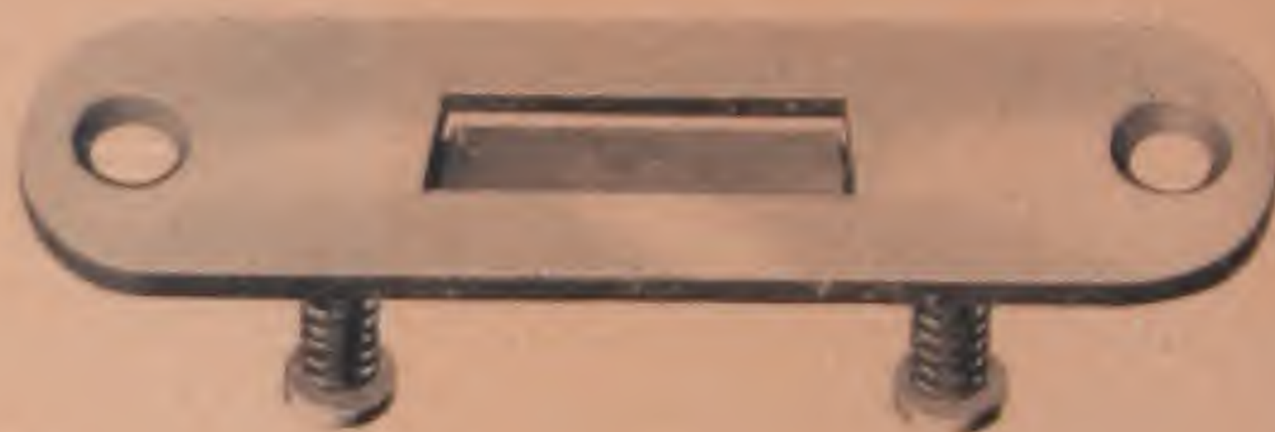
No. 321— 2\frac{1}{2} " x \frac{5}{8} " Self Closing Strike. Slot, \frac{1}{8} " x \frac{1}{4} ". Countersunk for No. 4 Screws.
